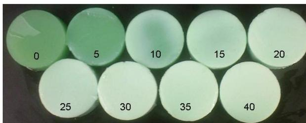
Fig 2. Photograph of albumen phantoms heated for different time periods. The number on each phantom represents the amount of time, in minutes, that each phantom was immersed in the water bath at 70°C
