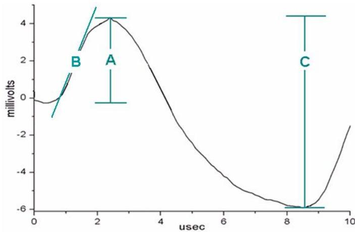
Fig 4. Typical photoacoustic signal denoting features: A - amplitude of the positive peak, B - the slope of the rising positive peak and C - signal peak to peak difference
