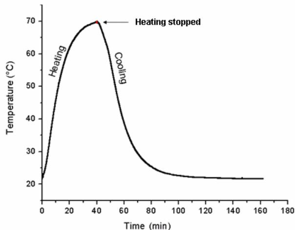
Fig 1. Temperature profile at the centre of an albumen phantom submerged in a 70°C water bath
