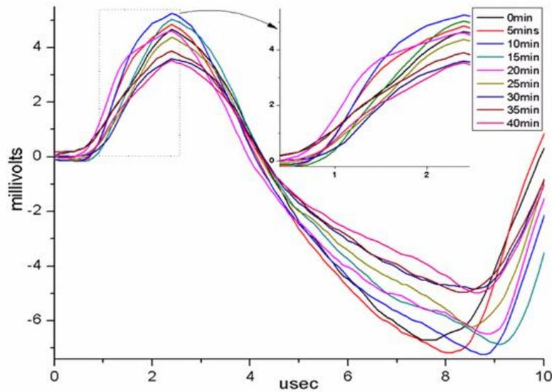
Fig 3. Averaged PA signals measured from tissue mimicking albumen phantoms as a function of heating time.
