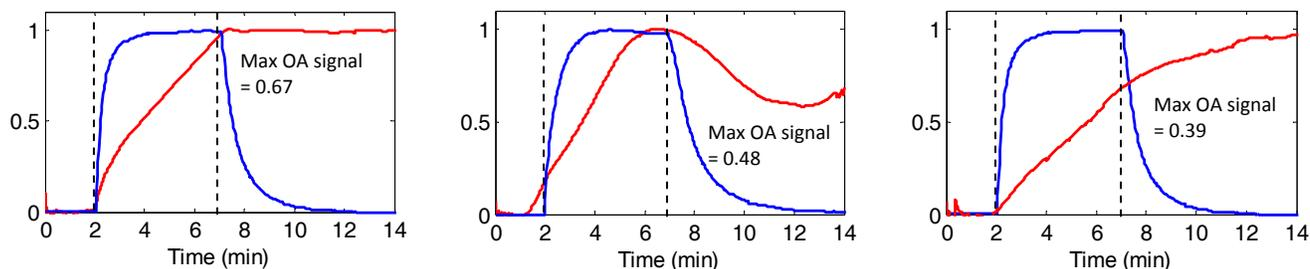
Figure 3: Normalized integrated OA signal (red) and normalized temperature measurements (blue) acquired 2 minutes prior to laser thermal therapy (LTT), 5 minutes during LTT and 7 minutes post LTT. Dashed lines represent begin and end of laser heating.
